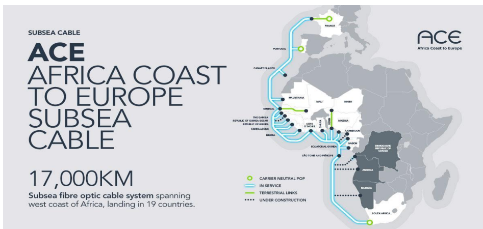
Figure 7: ACE subsea cable with a landing point under construction for Namibia
